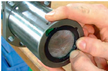
Fig. 4.7 Fixing the wiper while slowly screwing nut onto shaft
