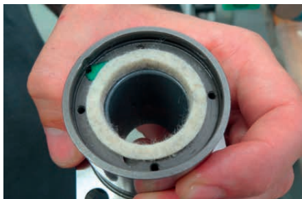
Fig. 4.12 Nut with inserted felt wiper
