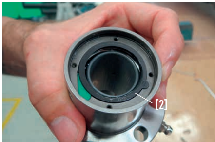
Fig. 4.13 NBR wiper [2] and support ring [1]
