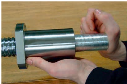
Fig. 4.6 Screw nut with wiper onto shaft
