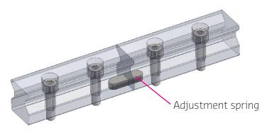
To simplify assembly, the rails can be supplied with a spring groove at the joint. The adjustment spring is recessed in the rail, the rails can be screwed directly onto a flat surface.
